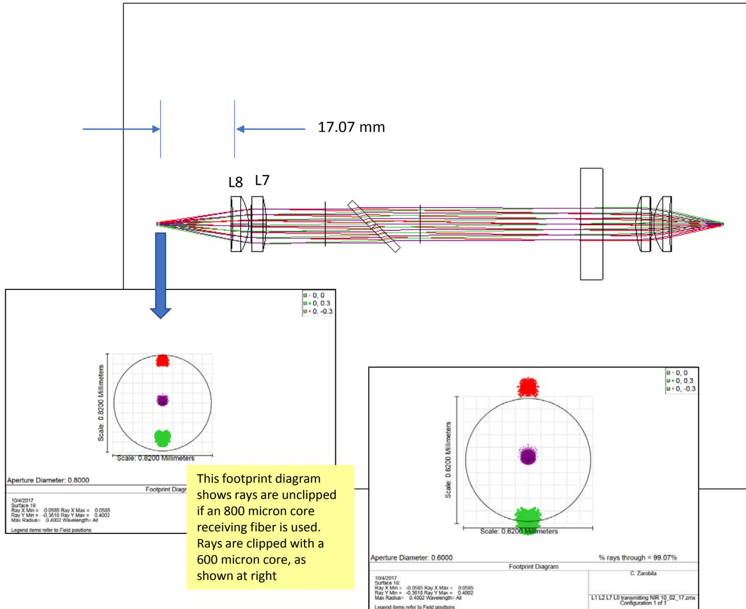
This footprint diagram shows rays are unclipped if an 800 micron core receiving fiber is used. Rays are clipped with a 600 micron core, as shown at right
