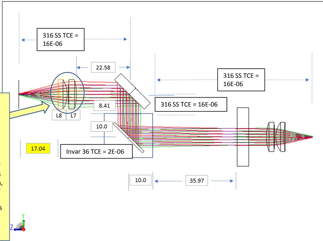
Worry that clear aperture of L7 is not large enough to pass all rays (non-sequential trace to be performed with parts in mounts). In transmitting path, distance from front of PDBS to L3 is about 24 mm; in reflecting path, distance from front of PSBS to L7 is about 41 mm. Although beam is collimated it still diverges so beam is bigger!
