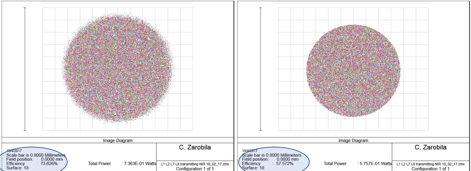
Expect about 22% less light to get through if using a 600 micron core fiber at the image plane vs. 800 micron core
