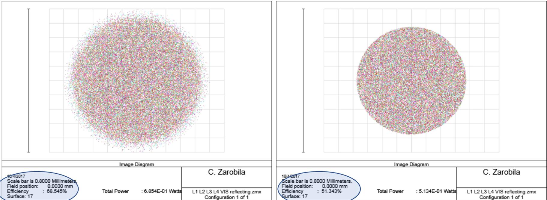
Expect about 25% less light to get through if using a 600 micron core fiber at the image plane vs. 800 micron core
