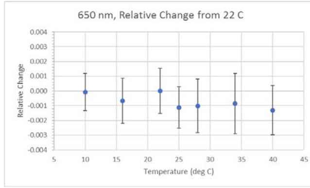
Sensitivity is worse, probably because of 600 micron receiving fiber. +/- 0.4 % contains all data including  $k = 2$  error bars
