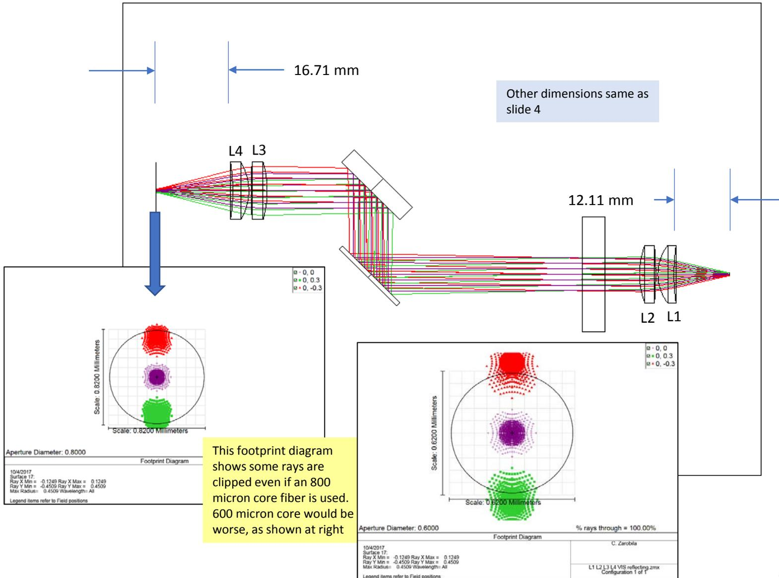
This footprint diagram shows some rays are clipped even if an 800 micron core fiber is used. 600 micron core would be worse, as shown at right
