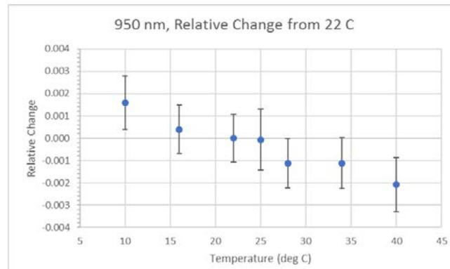
Sensitivity is worse, probably because of 600 micron receiving fiber. +/- 0.35 % contains all data including  $k = 2$  error bars
